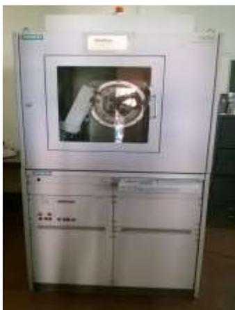
**Fig. 5.** X-ray diffraction (XRD) spectrometer.
