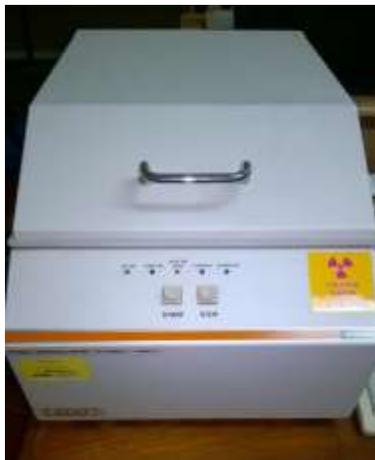
**Fig. 4.** X-ray fluorescence (XRF) spectrometer.
