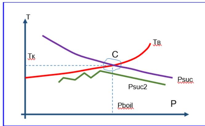
**Fig. 1.** Pump temperature vs. suction pressure (all other operating parameters remain unchanged).
