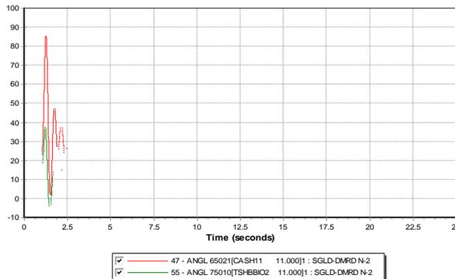
**Fig. 8.** Angle response when 132 kV Segaliud to Dam Road double circuit transmission lines are tripped.
