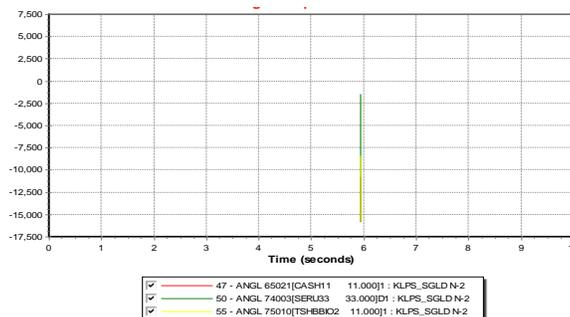
**Fig. 6.** Angle response when 275kV Kolopis to Segaliud double circuit transmission lines are tripped.
