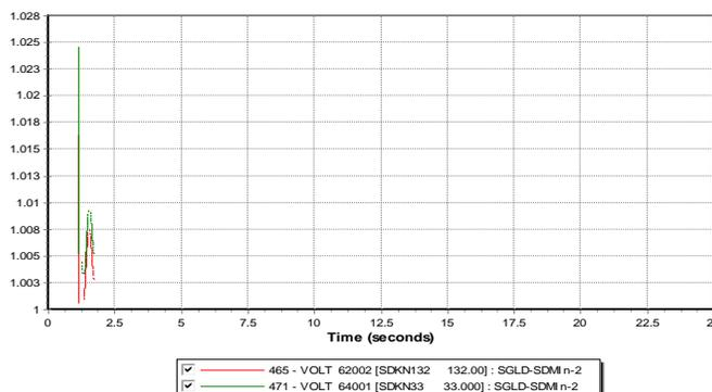
**Fig. 9.** Voltage response when 132kV Segaliud to Sandakan double circuit transmission lines are tripped.
