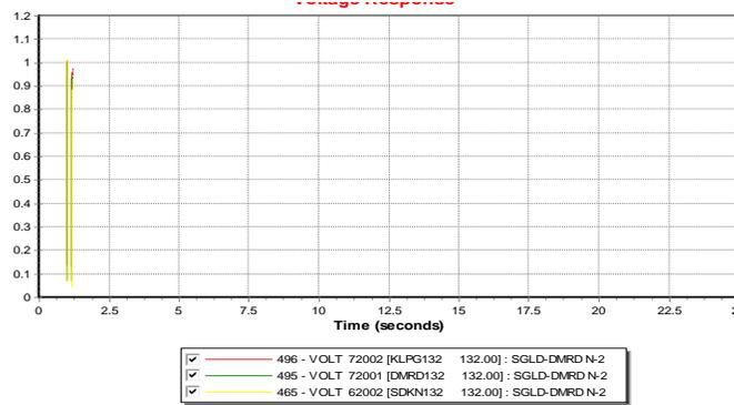
**Fig. 7.** Voltage response when 132kV Segaliud to Dam Road double circuit transmission lines are tripped.
