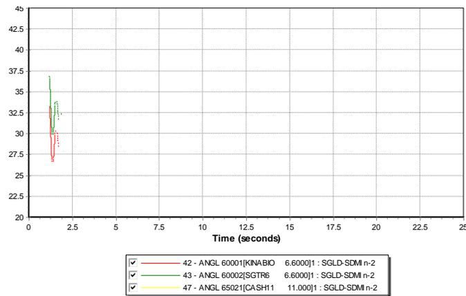
**Fig. 10.** Angle response when when 132kV Segaliud to Sandakan double circuit transmission lines are tripped.
