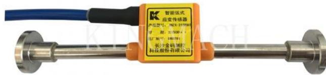
**Fig. 1.** JMZX-215 intelligent string-type digital strain gauge installed inside the bridge before casting.
