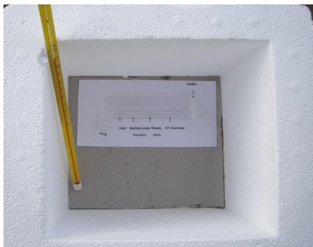
Fig. 8. Styrofoam box containing the HT microfluidic device and a thermometer
