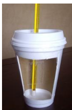
Fig. 7. Styrofoam cup containing the LT microfluidic device and a thermometer
