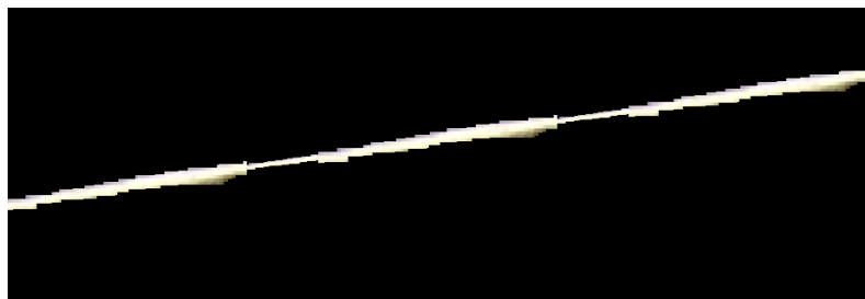
Fig. 7. Fancy yarn obtained using a roller with a segment
