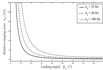
**Fig. 5.** The relative ranging error of different frequency shift measurement error.
