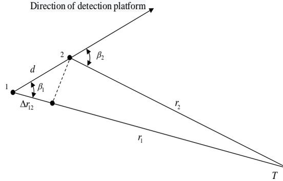
**Fig. 2.** Detection of fixed target by moving single station.
