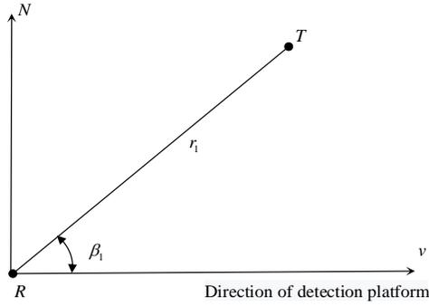
**Fig. 1.** Doppler frequency shift detection of moving single station.
